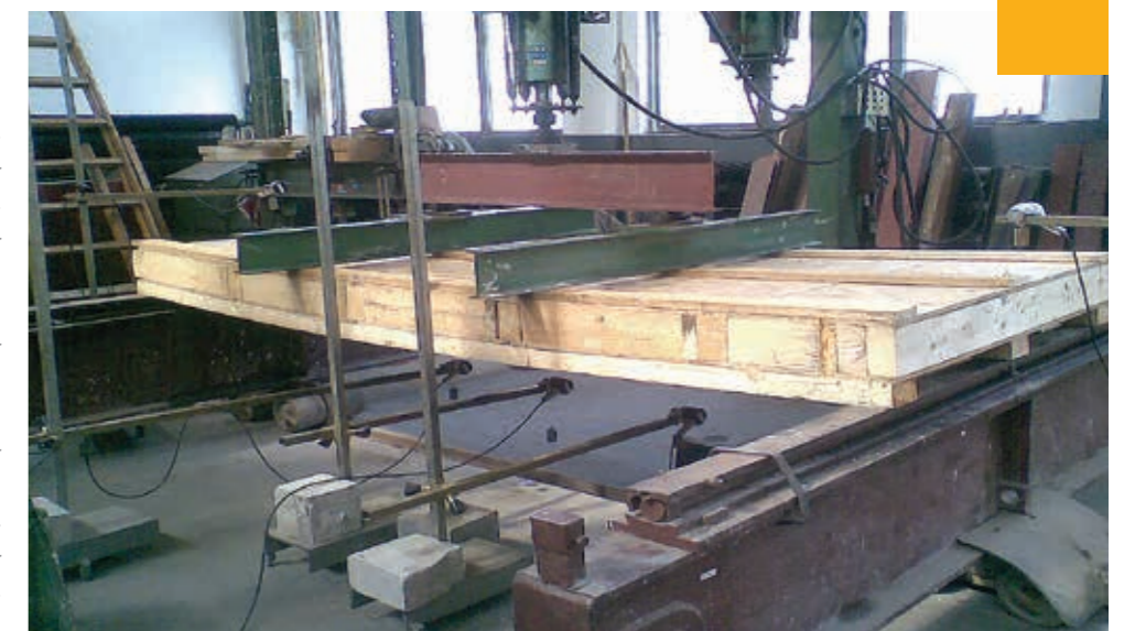
■ Skúška pevnosti v ohybe panelu na báze dreva EN 380 / Bending strength test of wood-based panel according to EN 380
