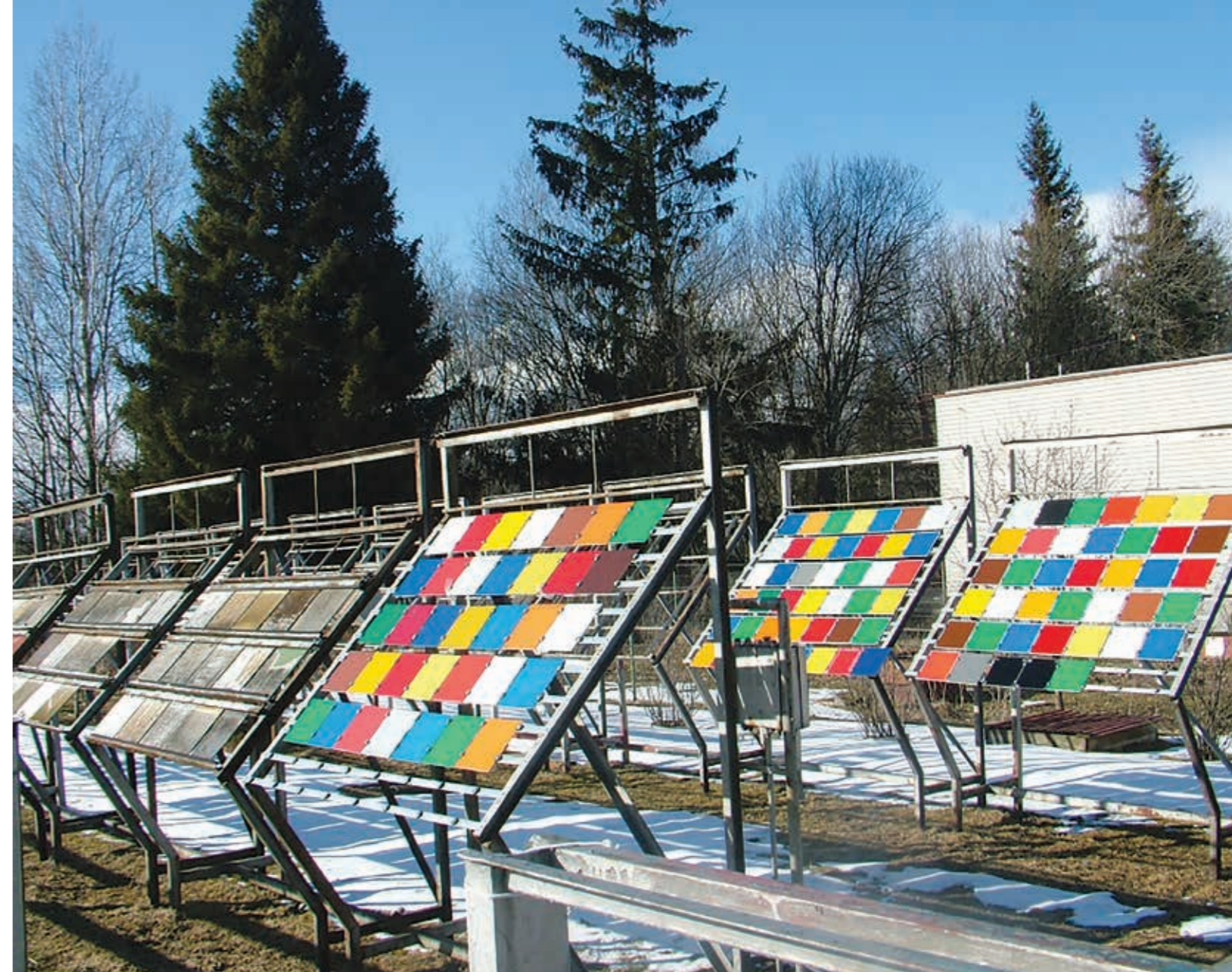
■ Expozičné stojany na klimatekovej stanici / Exposure stands at climate station
